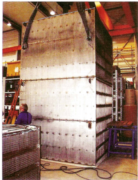
Fig. 11: Heating surface with 11 modules
